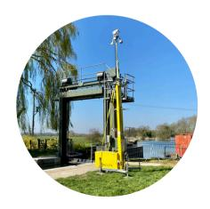
If your construction site has no power facilities, we would recommend using the Solar Fuel Cell Tower. The Solar Fuel Cell Tower is powered by a methanol fuel cell backed by a high-performance solar panel which reduces fuel consumption and increases the system's autonomous run time by up to 20 weeks before a refuel is required. The Solar Fuel Cell Tower is suitable for allyear-round usage, providing a reliable and consistent service even during those colder, darker seasons.
